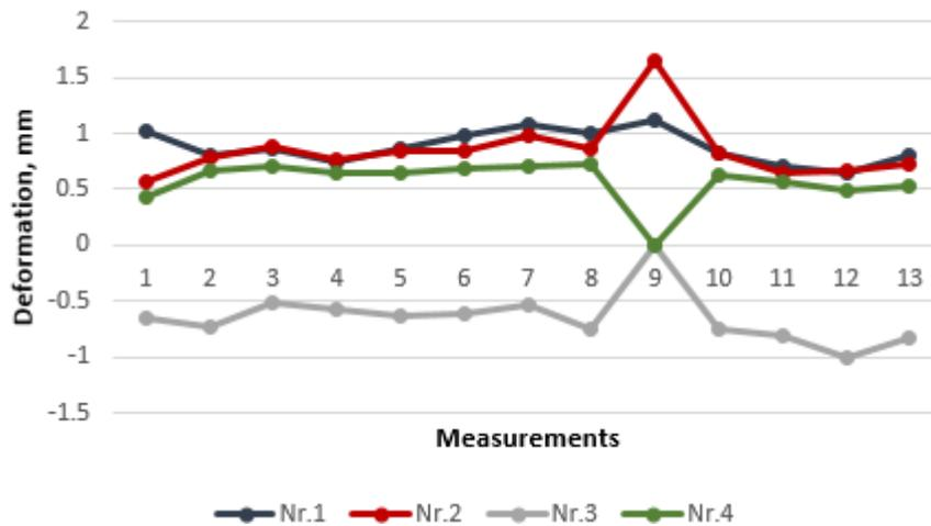
Fig. 8. Brick masonry deformation measurements
