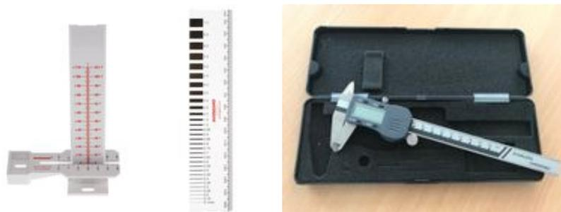
Fig. 2. Ruler sliding planes, crack width rulers and digital gauge (photo by J.Gruntmanis)
