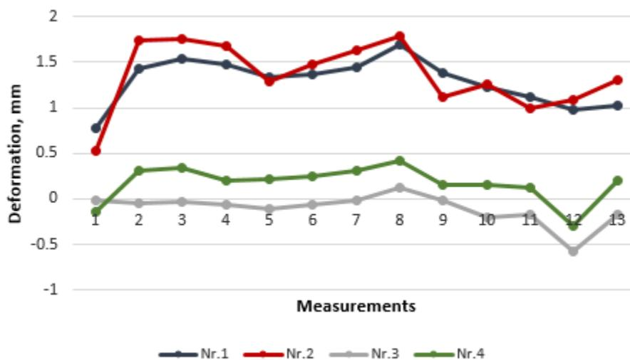
Fig. 7. Aeoroc (aerated concrete block) masonry deformation measurements
